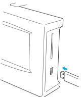
When connecting the USB Card Reader/Writer to the machine's USB Type "A" (host) port, be sure to secure the cable with the three hooks on the back panel. If the cable is not secured, the embroidery frame may catch on the cable while the frame is moving, causing the pattern to become misaligned.
